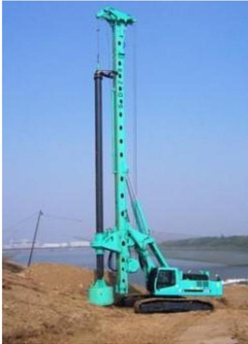
Noise reduction measures including use of pile drilling instead of pile driving where possible
